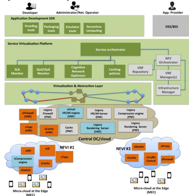
FIGURE 1. HIGH-LEVEL ARCHITECTURE OF THE 5G-MEDIA PLATFORM
